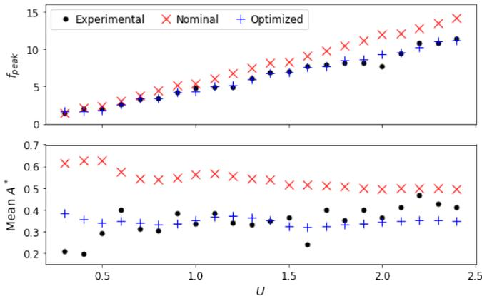
Fig. 7 Comparison of spatial average displacement  $\overline{A^*}$  among experimental result (black dot), nominal VIVA prediction (red cross), and VIVA prediction with optimal hydrodynamic database for NDP 38m experiment in linearly sheared flow over different maximum incoming velocity  $U$  in a unit of  $m/s$ .
