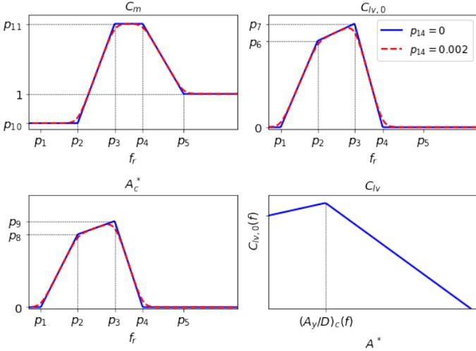
Fig. 8 Parametric model for the hydrodynamic database.
