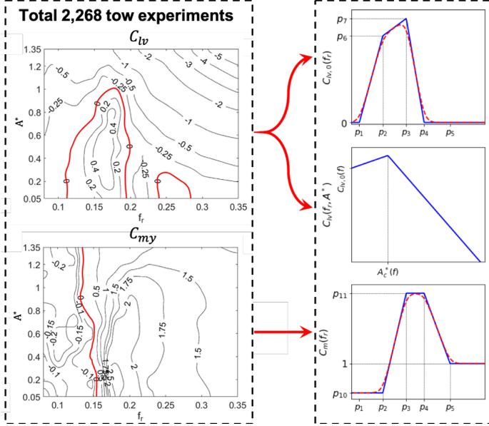
Fig. 1 The simplification of a hydrodynamic coefficient database constructed by a large number of rigid forced vibration experiments (left) (Fan *et al.*, 2019(2)), using simple piecewise linear models with a set of parameters to be learned from the data (right).
