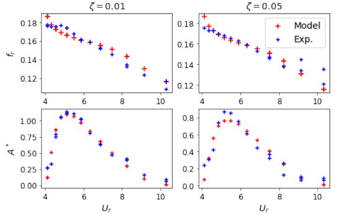
Fig. 3 Comparison between experimental result (blue) and model prediction (red) of frequency (first row) and amplitude (second row) response for different damping ratios:  $\zeta = 0.01$  (right column) and  $\zeta = 0.05$  (left column).
