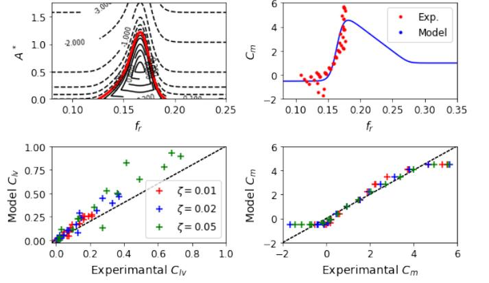
Fig. 2 Learned optimal hydrodynamic database of  $C_{lv}$  (left column) and  $C_{my}$  (right column). The second row shows the correlation between the experimental measurement and learned parametric model predicted hydrodynamic coefficients.
