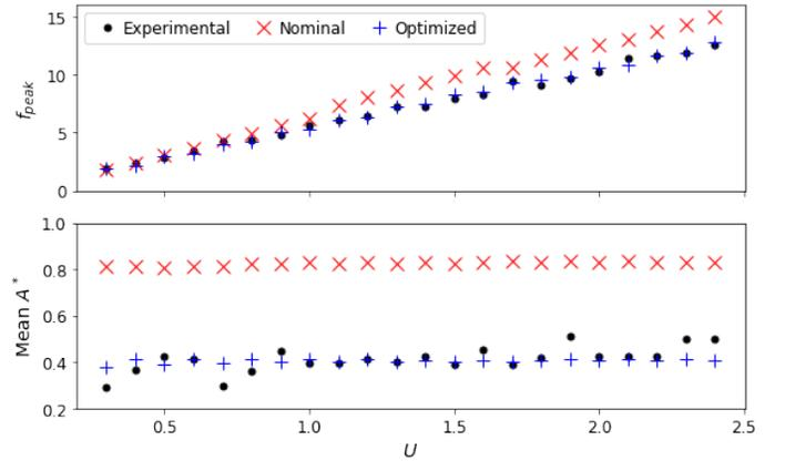
Fig. 6 Comparison of spatial average displacement  $\bar{A}^*$  among experimental result (black dot), nominal VIVA prediction (red cross), and VIVA prediction with optimal hydrodynamic database for NDP 38m experiment in uniform flow over different incoming velocity  $U$  in a unit of  $m/s$ .
